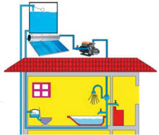
Hot water boosting in solar heating system
