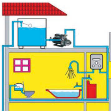
Indirect roof tank water pressure boosting
