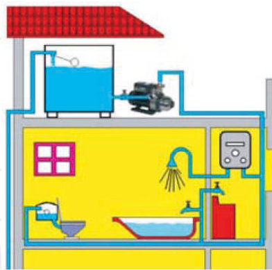
Indirect roof tank water pressure boosting
