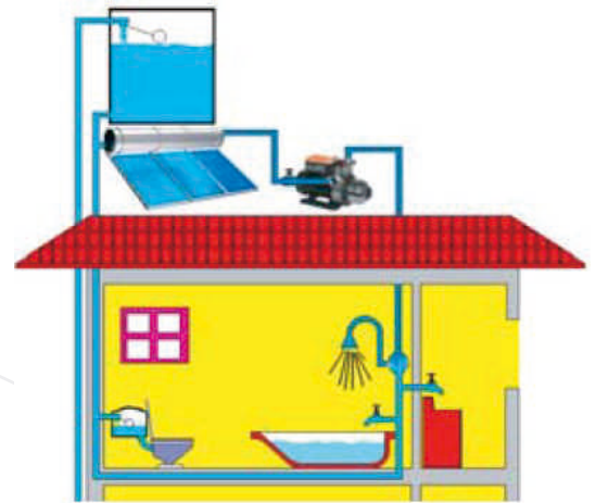
Hot water boosting in solar heating system
